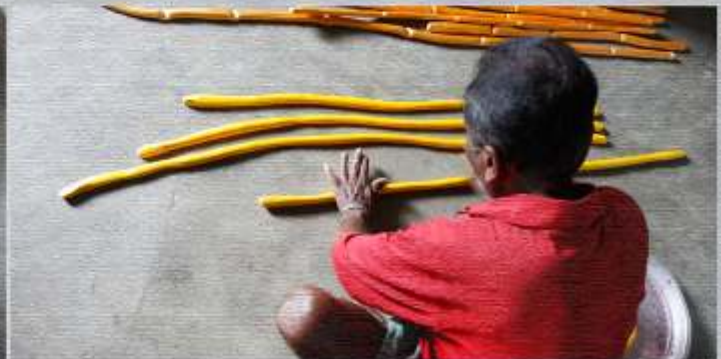
It is then kneaded and made into long rods and cut into small lac sticks before it hardens. The lac sticks are then used to colour and coat the wood.
