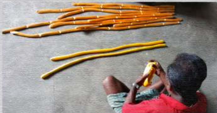
It is then kneaded and made into long rods and cut into small lac sticks before it hardens. The lac sticks are then used to colour and coat the wood.
